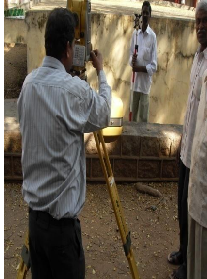
Total Station Survey
